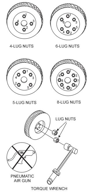
Figure 4. Wheel Lug Nuts Tightening Sequence
